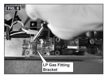
8. Remove solenoid valve retainer (bracket) with its two mounting screws, and discard. See FIG. 9.
