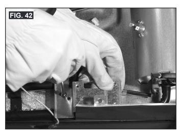
16. Reinstall burner housing with solenoid valve and complete burner with its three mounting screws. Then reinstall LP gas fitting bracket with its two mounting screws. See FIG. 43.
