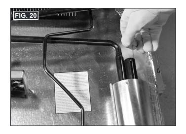
23. Remove OLD thermodisc from cooling unit. Then remove OLD thermodisc from wires and discard. See FIG. 21.
