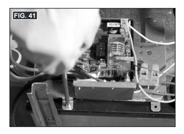
15. Install NEW solenoid valve retainer (bracket) with the two NEW screws provided. Do not tighten screws to allow slack. See FIG. 42.
