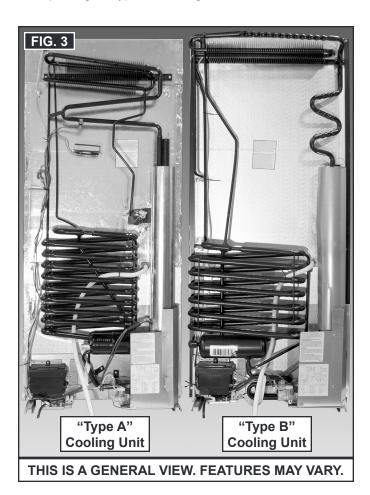
C. Removal Of "Type A" Cooling Unit
