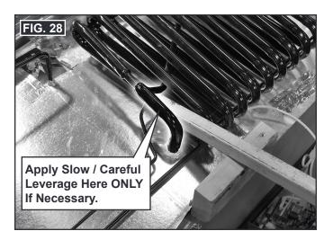
30. Continue to lift off the OLD cooling unit completely. See FIG. 29.
