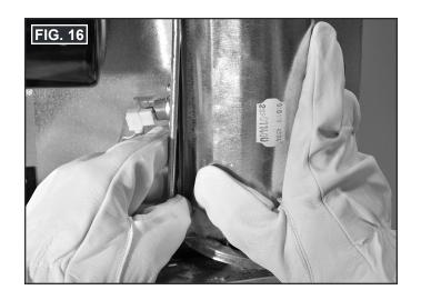
19. Continue to separate seam approximately 6" above heating element. See FIG. 17.
