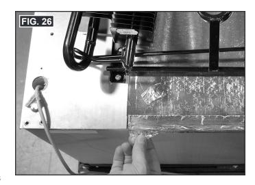
29. Lift the OLD cooling unit and carefully guide the conductor (cable) through the top bracket hole. Allow conductor (cable) to hang freely from the refrigerator cabinet. See FIG. 27.
