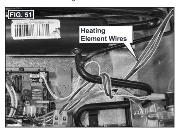
27. Route conductor (cable) under cooling unit and reconnect to power module's circuit board terminal P1 (top left plug). See FIG. 52.
