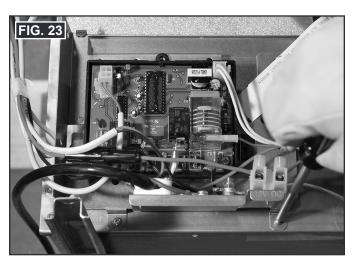
26. Remove four frame screws from top bracket and remaining two screws from bottom plate. Save screws for reinstallation. See FIG. 24.
