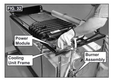
Route the conductor (cable) near the top of the refrigerator behind the cooling unit piping, and reapply insulating putty around cable and fill hole. See FIG. 33.
