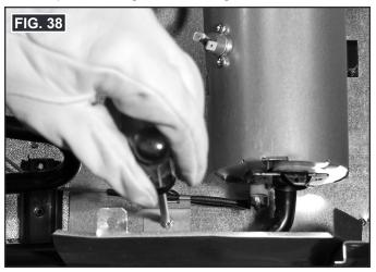
12. Reinstall three hex head drill point screws attaching cooling unit frame to refrigerator. Two screws at top, and one screw at bottom left. See FIG. 39.
