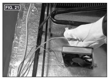
24. Remove fan from back of cabinet, and allow to hang freely out of the way. Discard fan bracket with its two mounting screws. See FIG. 22.
