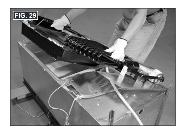
31. Remove cooling fins with its four mounting screws from the OLD cooling unit, and save for reinstallation. Discard OLD cooling unit. See FIG. 30.
